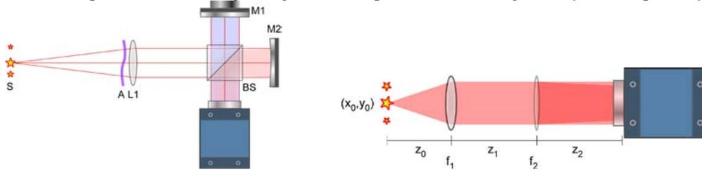
Fig. 1: a) Interferometer for incoherent digital holography; b) geometry of the optical configuration.
